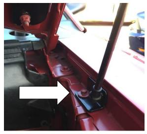
3. Install the Hood Brackets. Using a 10mm socket, remove the most forward nut completely. Loosen the rear hood nut to allow the Hood Bracket to fit between the hinge and the nut, NOT, between the hinge and the hood. Note: For ease of installation, the Hood bracket is slotted so the rear nut does not need to be removed completely. Position bracket as shown, replace the forward nut, and tighten both nuts.
