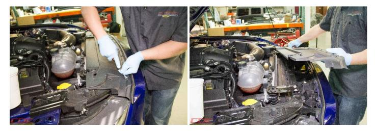
6. Remove the (2) 5.5mm bolts at the corners of the Fascia, located near the Headlights under the rubber Hood Seal.
