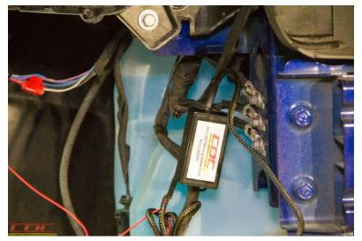
18. Place Fascia close to the Car and plug in the Drivers to the LED's. Test the function of the Outlaw Grille Lights. **Note**: The AutoDim feature (dims the DRL's about 40% when the Headlights are on), requires the car to be running.
