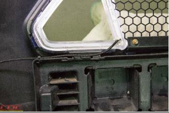
15. Plug the Plug and Play Harnesses into the Turn Signal Connectors and secure wires with Zip Ties as shown.
