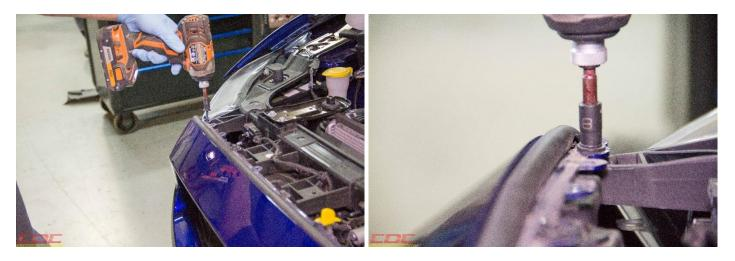
8. Remove the Plastic Retainers and 7mm bolts that secure the Splash Shield to the bottom side of the car.
