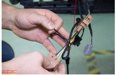
16. OPTIONAL: Connect the AutoDim (RED) wires. Strip back approximately 2"-3" of the black wire loom of the Headlight wiring Harness (be very cautious not to damage any wires). Locate the GREY with PURPLE stripe wire. Use the provide Inline splicer to connect the RED Pigtail Wire to the Grey with Purple stripe wire. Use the provided Silicon Dielectric Compound to seal the conectors. Zip Tie the wire to the RED wire to the Headlight Harness, and trim excess Zip Tie.
