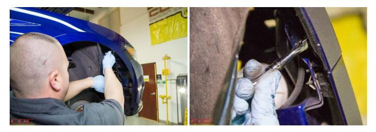
5. Remove Radiator Cover. Remove all the Plastic Retainers, and remove Cover from vehicle.
