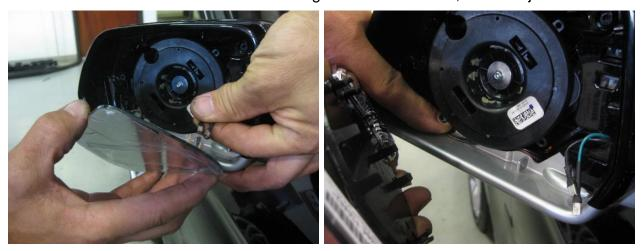
11. Align plastic retainers to adjuster, and gently push until all the fasteners engage.
