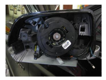
9. Reinstall outer ring with screws previously removed. Plug in Signal Mirror at this time.
