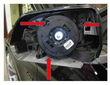
6. Disconnect connector as shown below, and set adjuster aside.
