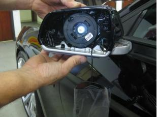
10. Connect heater wires to mirror. Route Signal wires as shown, below adjuster.
