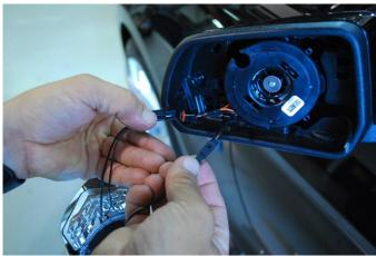
10. Connect heater wires to mirror. Route Signal wires as shown, below adjuster.
