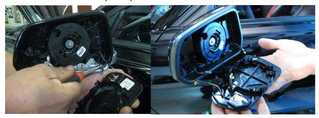
3. Remove the (2) T-15 screws that secure the outer ring to the mirror housing. Use small Screwdriver to release clips, and remove outer ring.
