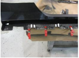
10. Using the holes in the Outlaw Rockers as drill guides, drill 3/16" holes as shown and install the supplied 3/16" rivets, and rivet washers.
