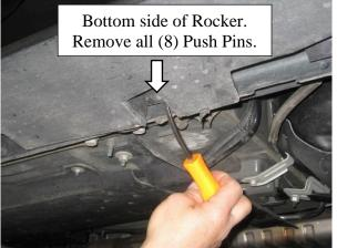
6. Starting at the rear, pull the Rocker away from the vehicle to gain access to the Rocker Clips that secure the top edge of the rocker to the body. Use a Panel Tool to help disengage the clips. You will inevitably break some clips, but don't worry we have included new clips to install your CDC Outlaw Rockers. Remove the remains of any broken clips, and discard. CAUTION: Careful not to damage painted surfaces while prying with Panel Tool, apply masking tape to the areas if necessary.
