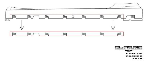
9. Attach lower portion of stock Rocker to your CDC Outlaw Rocker. Align the part with the openings on the Outlaw Rocker and hold to the edge of the Rocker. Use spring clamps or similar to temporarily hold in place.
