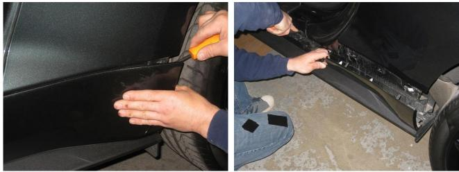
7. Remove Aero Deflector from stock Rocker. Remove the T-27 screws and "J" Clips (will be installed on your Outlaw Rocker).
