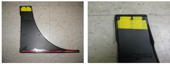
2. Assemble the Winglets to the Outlaw Rockers. <u>Note:</u> The Winglets are separate to make the painting process easier. The parts are pre-taped with 3M VHB tape. Remove the Masking tape from the back side of the Winglets, clean with the area with the supplied Alcohol Pack, and allow to dry. Apply the supplied Adhesion Promoter and allow to dry. Peel the red backing from the tape, use the alignment pins to locate the parts, and press the parts together firmly.
