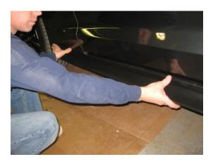
15. **OPTIONAL, BUT HIGHLY RECOMMENDED:** Apply a bead of silicon where Winglets meet the Rocker, to avoid debris and water from collecting. Apply masking tape as shown, apply a small bead, and wipe in a nice fillet with fingertip. Peel masking tape.
