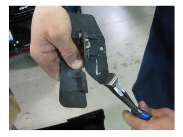
12. Install the Aero Deflector (removed from stock Rockers in step # 3) on the Outlaw Rockers. Install the "J" clips, and the T-27 screws.
