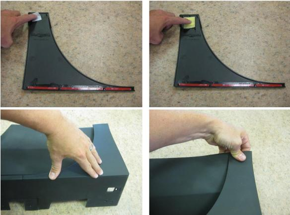
3. Melt the 3 locator pins at the top of the Rockers with a soldering iron or similar as shown below.
