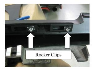
14. Install the Outlaw Rockers. Starting at the front, align the Rocker Clips and snap into place. Reinstall the Push Pin fasteners in the wheel openings and the underside.
