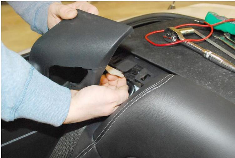
**WARNING:** Make sure trim panels are tucked in behind the convertible top as shown below. Damage will occur to the trim panel when top is cycled if this is overlooked.
