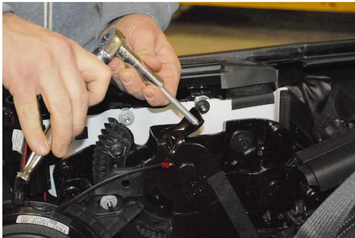
Supplied Cut Off switch pictured below. Used to "break the ground" when the convertible top is up so that the LED brake light in the CDC Lightbar is disabled. Adjust jamb nut to measurement in step #20.
