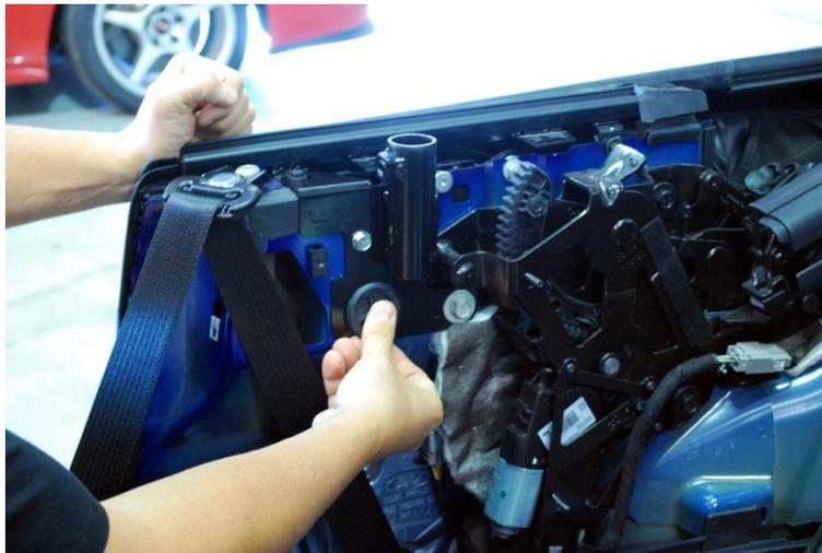
18. Install provided Lightbar wiring harness. Feed connector up through the bottom side of the receiver tube of the bracket, and bend wires over as shown in picture below. (Bending the wire over will temporarily hold the harness in place.)
