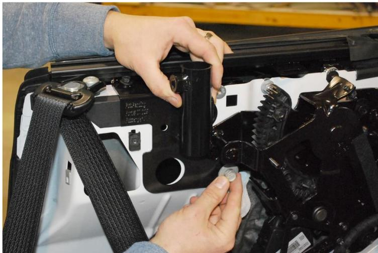
Install the provided 5/16" Button Head bolt through the hole in the center of the bracket and the pre-existing hole in the vehicle.
