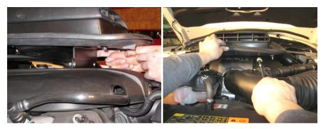
4. Attach the Air tube Adapter to the Upper Air tube. Do not tighten at this time.
