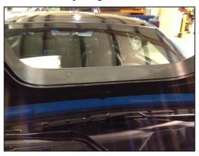
8. There are two 3/32" holes that are predrilled in the front and rear of the Upper Ring (4 total), and two sets of holes (upper and lower) drilled into the Lower Ring (8 total). Use #183011 rivets to secure the Upper and Lower Trim Rings together, using the UPPER holes in the Lower Trim Ring.
