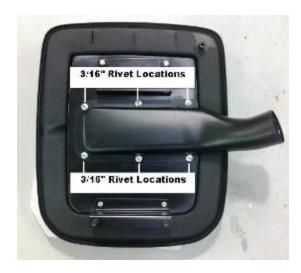
2. Install the Shaker Assembly. Slide the air tube adapter over the lower airtube with both clamps loosely, at this time.
