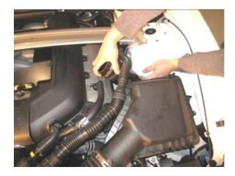
3. Align the ball studs with the receivers and firmly press on top of scoop. You should feel the scoop pop in to place. After the ball studs are engaged, pull the Shaker assembly forward so that the front mounting bracket is in front of Manifold bracket. Now align the 2 front mounting holes and install the M6-1.0 x22mm bolts. Hint: Put a small piece of masking tape in the socket to help hold the bolt.
