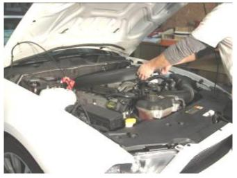
6. Remove Air Box. Release the 2 clips that secure the lid. Loosen the hose clamp (8mm); disconnect the Mass Air Flow Sensor Connector. Remove the sound tube mount from airbox, and finally remove the 10mm bolt securing the lower air box near the fender.
