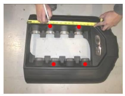
2. Drill the 4 locations. Start with pilot hole, then enlarge with 3/4" to 1" step bit or hole saw. Note: You will start your hole approximately 1/8" from the angled wall of the engine cover. When you drill the 3/4" to 1" hole, you will be drilling the flat surface and the angled surface.
