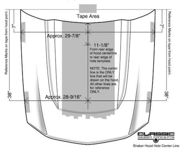
9. **2011-2012:** On the centerline, measure 11½" from rear of the hood and mark a line on the tape, intersecting the centerline. This will align with the rear cutout line of the Shaker Cutout Template.
