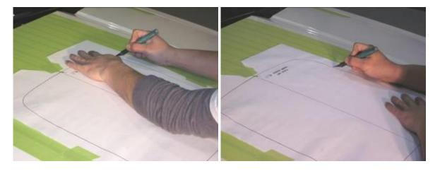
14. Remove Template from hood and discard. Peel tape from center of Shaker opening, leaving an outline of Shaker opening.
