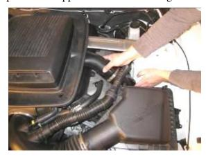
5. Install Drain tube and route safely, away from pulleys, exhaust manifold, etc.
