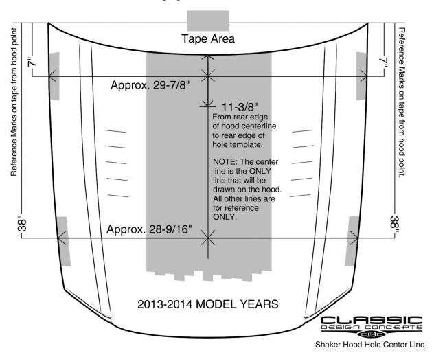
11. **2013:** On the centerline, measure **11-3/8**" from rear of the hood and mark a line on the tape, intersecting the centerline. This will align with the rear cutout line of the Shaker Cutout Template.
