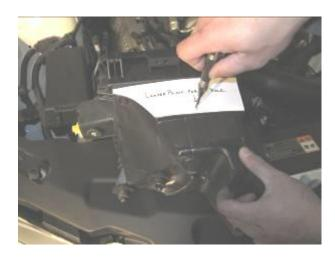
2. Remove the paper template and carefully drill the hole with a 3" hole saw.
