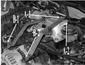
Note: Torque ball studs to 40 inch pounds, over tightening will damage ball stud.
