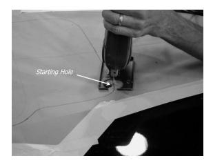
G) Place Appliqué on hood to verify hole locations and fitment. Open holes as necessary to obtain proper fitment. Remove Applique' once desired located is achieved.
