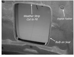
Note: Bulb on seal should be on outside of opening.
