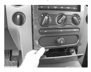
Note: Use care when pulling on the bezel, the clips are difficult to dislodge. Be careful not to over bend the stack causing a crack.
