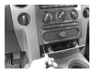
2. Grasp the center stack bezel and pull outward to dislodge clips.
