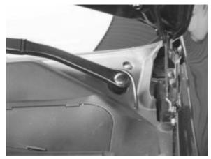
D) Route the Driver Side Hose (63") toward the center of the engine bay.
