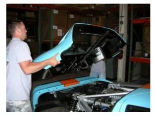
**3.** Remove Air Box to gain access to exhaust tip clamps. Loosen the 8mm hose clamp. Unplug Mass Air Sensor. Remove the (2) 10mm mounting blots. Remove Air Box from vehicle.
