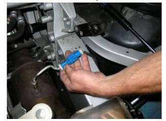
**9. Remove Ground Wires from Horns**. Remove the 10 mm bolts that secure the ground wires on both Frame Horns.
