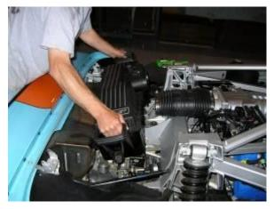
**4. Remove both Rear Fascia Closeout Panels.** Remove the push pin fasteners and Scrivets. (6 New push pins included in kit for reassembly)
