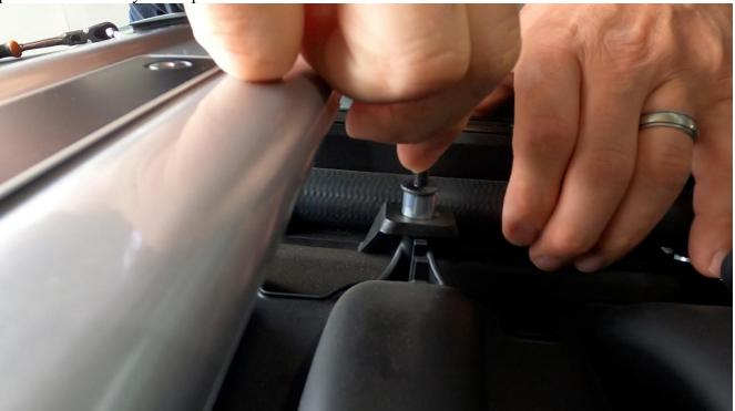
33. On the passenger front stud place a spacer #57002 (.482") on top of the stud flange.
