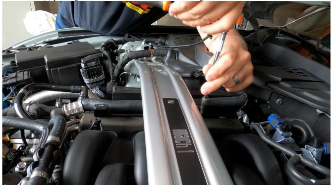
31. Replace the passenger front stud bolt on top of the "Powered by Ford" part and WITHOUT a spacer between the plastic "Powered by Ford" part and the stud bolt.
