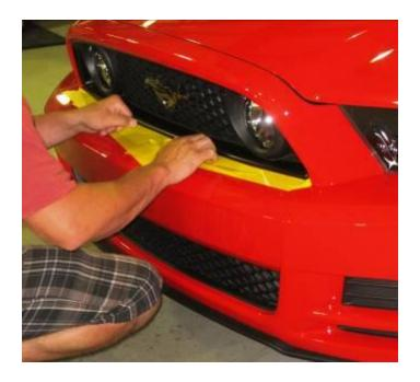
2. Remove factory Grille. Firmly grasp Grille just inboard of the Fog lights. In a swift motion, pull grille to dislodge the surrounding clips.
