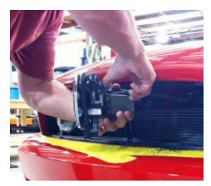
4. Secure wiring harness. Wrap the ends of the wiring connectors with electrical tape to keep out debris. Fold the harness and secure with the provided Zip Ties as shown in pics.
