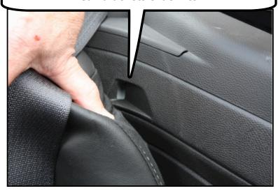
Standing on the drivers side. Flip out the rear bracket on the passenger end. This is what will slide into the slot beside the back seat on the passenger side.
