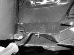
5. Remove the downward screws securing the ends of the factory trim piece to the fascia (1 per side).
