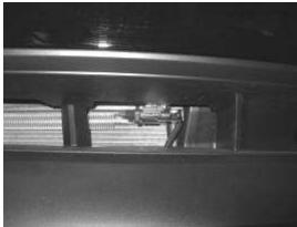
19. Re-install the factory slash shield with the factory fasteners.
