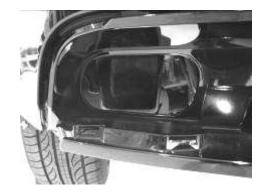
11. Install factory J-Clips, removed in step #8, onto the CDC Chin Spoiler. Note orientation of clip.
