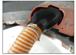
8. Route tubing behind plastic wheel well liner and along sway bar; secure to sway bar using the supplied zip ties. Route outward to brake area.
