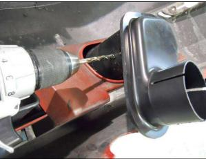
5. As an option, you may also drill from the top side of the driver duct and far right side of passenger duct, but only one push-pin is absolutely necessary.
