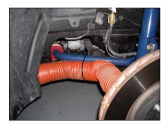
9. Remove the two primary caliper anchor bolts, and support the caliper so that it is not hanging on its brake line.
