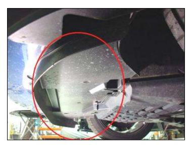
3. With CDC/RTR Chin Spoiler already installed onto vehicle, install CDC brake duct adapters from under the vehicle. Push ducts all the way onto chin until they stop. Note that passenger-side adapter is designed to extend around windshield washer reservoir.
