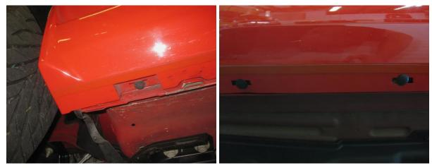
5. Apply Adhesion Promoter to Splitter as shown in pic. **NOTE:** Apply Promoter where tape will contact the Splitter.
