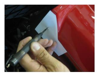
9. Drill both front and rear locations with ¼" drill. **NOTE:** If you did not jack the car up, you will need a right angle, or 90 degree drill. It's ok if you drill through the 3M tape.
