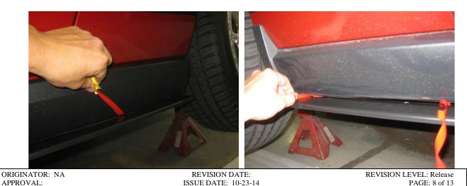
8. Using the Splitter as a drill guide, drill the remaining  $\frac{1}{4}$ " holes and install push pins. Repeat the process on the opposite side of the car.
