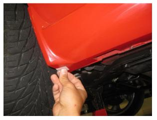
3. Apply the supplied Adhesion Promoter to bottom side of the Rocker Panel. Allow sufficient time to dry.
