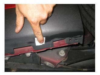
2. Apply Adhesion Promoter to the bottom side of the Rocker as shown. Allow sufficient time to dry.
