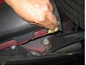
3. Apply 3M tape to bottom side of Rocker. **NOTE:** Use the rectangle cutouts in the bottom of the Rocker as a guide to place the 3M tape.
