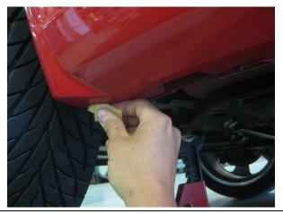
4. Apply the 3M tape as shown below. **NOTE:** Apply the tape approximately 1/16" inboard of the corner of the Rocker Panel.
