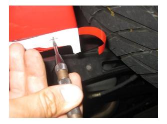
8. Align template as shown at front of Rocker. Mark the Rocker with a center punch.
