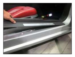
3. Remove the 2-piece passenger kick-panel plastic covers, exposing wire harnesses. Pull rear-ward on large portion of kick panel to dislodge clips.
