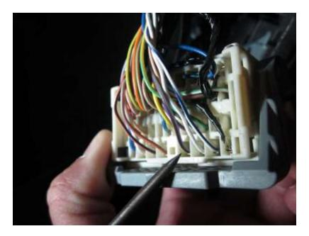
This wire will feed the positive side (red wire) of the iLight. A few inches from this large connector, attach a red T-Tap (provided) connector to this Gray/Purple stripe wire, closing the T-Tap firmly with pliers.
