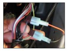
15. Reinstall gray connector to SJB, reinstall kick panel and door sill, resume remainder of Lightbar installation.
