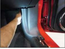
4. From the Lightbar bracket, route iLight wire harness downward behind the plastic trim panel and forward toward the passenger kick panel area. Route the harness along the existing body harness (behind the carpet) and secure with electrical tape or plastic zip ties. Be sure the wire will not chafe or get pinched along any sharp metal edges.
