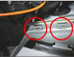
13. Carefully maneuver SJB around to access back panel, locate top gray electrical connector and disconnect carefully by depressing lock and pivoting arm. Pictures on following page.
