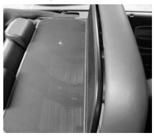
B) There is a small T-10 Torx Head Setscrew at the hinge on each end. Adjust this setscrew to limit the forward travel of windscreen to maintain the  $\frac{1}{2}$  gap.
