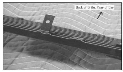
17. Place Billet Grille onto fascia and start all six mounting screws through Grille Mount Tabs into brackets, use thread locker on all screws. Just snug screws at this time.
