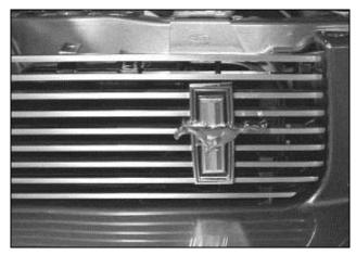
19. Tighten all mounting screws at this time. **Caution! DO NOT OVERTIGHTEN SCREWS!**
