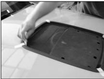
F) With the hood blanket on the bench, line up the Lower Trim Ring (part # 115050) with the line traced from the upper. Now trace the outside of the Lower Trim Ring onto the hood blanket. Note: Trim Ring will follow contour of the hood blanket when properly positioned, the hump is toward the rear. Remove Lower Trim Ring and measure 1/2" from the outer line toward the center of the hood blanket and mark one more line, this is the line you will cut using a sharp blade. Cut out blanket.
