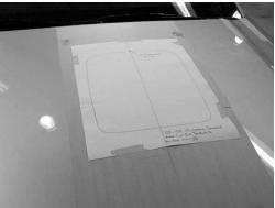
E) With a sharp razor blade or x-acto knife cut through template, through the tape, and into the paint of your hood along the cut-out line. Cutting/scoring the paint on the hood will reduce the chance of paint flake during the cutting process.
