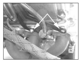
F) Trim the factory bracket with a cut-off wheel or hack saw. Follow lower horizontal line of the "FoMoCo" logo. Paint the cut area to prevent rust. (See figure below)
