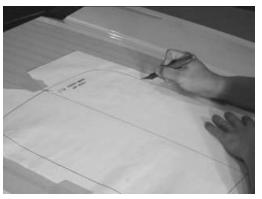
F) Remove template from hood and discard. Peel tape from center of Shaker opening, leaving an outline of Shaker opening. **CAUTION:** Add a second layer of tape around opening to reduce the risk of shavings scratching the hood.
