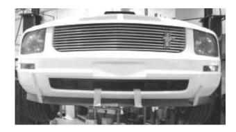
6. Using the Chin Spoiler fastener holes as a guide, drill the 10 fastener holes into the fascia.
