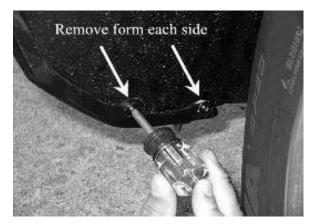
4. Attach both ends of Chin Spoiler at wheel openings with the factory screws removed in step #3.
