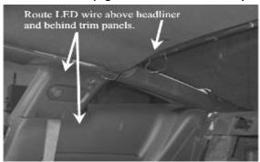
7. Pull Upper Quarter Trim Panel loose from sheet metal, but do not remove, for the routing of Brake Light wire. Route the Brake Light wire above the headliner and down behind both the Upper and Lower Trim Panels
