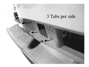
2. For the best overall appearance of your vehicle, we recommend that you black out the outer perimeter as well as the areas behind the lower Grille with Flat Back paint. Tape off fascia along the Inner/Second Feature Line from front (see picture below). Place the CDC Lower Grille into position on vehicle to verify where tape line should be. Tape large enough area to protect painted surfaces around the Grille Opening. Scuff surfaces to increase adhesion of paint.
