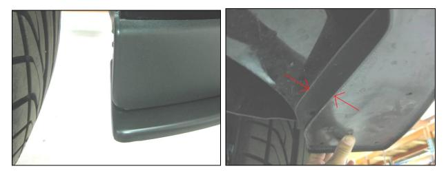
4. Looking down from above, "overhang" of Chin Splitter should be evenly spaced around Classic GT Chin; approx 7/8" at either end, and 1.25" at the front/center.
