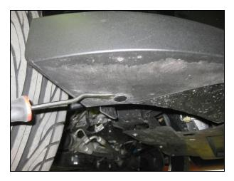
3. With spring clamps nearby within reach, place Chin Splitter to underside of the Classic Chin Spoiler and clamp in place. It helps to have a friend assisting. Left/right ends of Chin Splitter should fit flush with ends of Classic GT Chin Spoiler. Underside of Chin Splitter matches/overlaps contours of Classic GT Chin.
