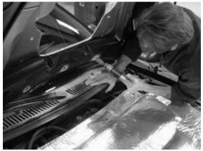
Note: DO NOT DRILL THROUGH THE HOOD OUTER WITH HOLE SAW!
