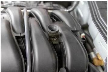
C) Loosen the (2) upper Throttle Body bolts (8 mm), but do not remove.
