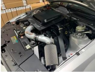
D) Install Drain Hose. Safely route hose away from any extreme and moving engine parts.
