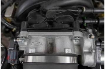
D) Install Shaker assembly. Push the Ball Stud into the rubber Ball Stud socket receiver, previously installed on manifold. Next, align the Throttle Body bracket (front of Shaker assy.) onto the Throttle Body bolts, loosened in previous step.
